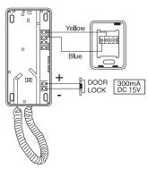
You should connect the wires as shown on the drawing
