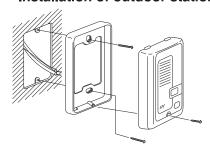
After attaching the body supporter with 2screws,put the Door Camera into the grooves of body supporter, and then fix it with screws.
