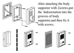
Outdoor station can be attached on a wall or on a door as shown on the drawing.
